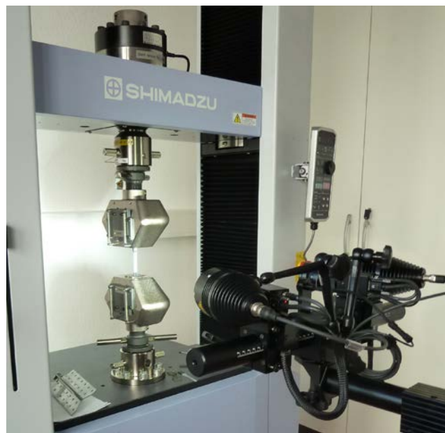
Fig.1: Tensile testing equipment and optical measurement system by GOM ARAMIS.
