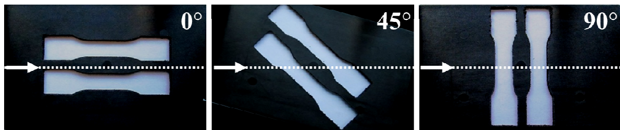
Fig. 1: Specimen cutting orientations relative to the flow-induced fiber direction (arrows).
