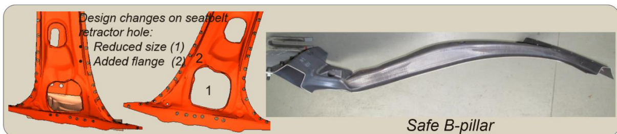
Fig.13: Improved B-pillar with safe lower area thanks to design modifications.
