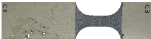
Fig.6: Example of tensile specimen (spokes) presenting some pores due to the casting process.
