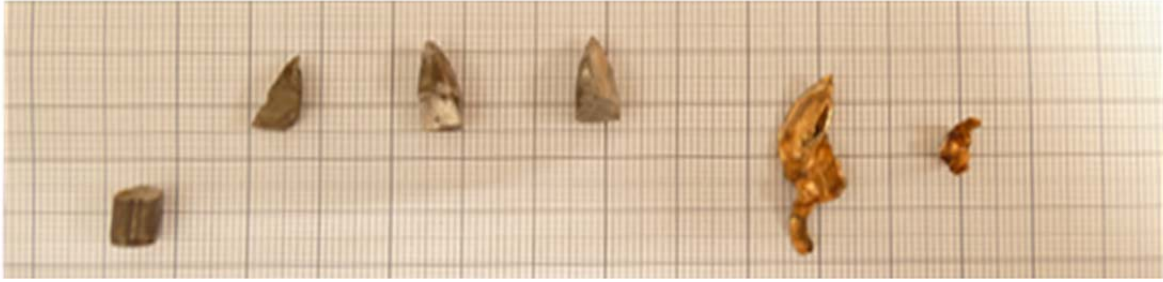
Fig. 5 Projectile parts retrieved after oblique impact, core and jacket
