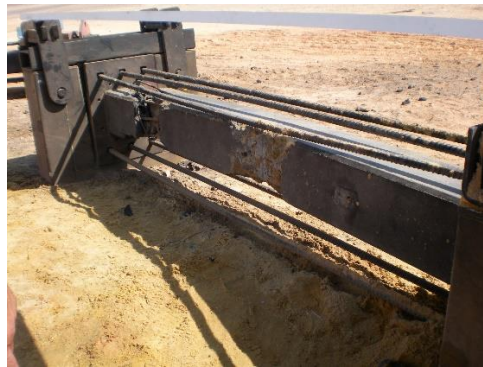
Fig.11: Damaged Test Column
