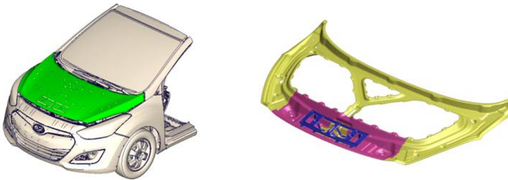
Fig.12: Load case hood closing analysis: finite element model (left), extra part definition at the inner panel in order to evaluate the stress due to hood closing (right).
