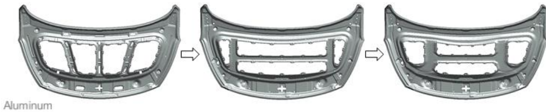
Fig.20: Initial design (left), design after topometry optimization (center) and design after shape optimization (right) of the inner aluminum panel.
