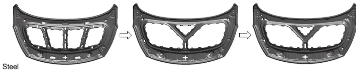
Fig.18: Initial design (left), design after topometry optimization (center) and design after shape optimization (right) of the inner steel panel.
