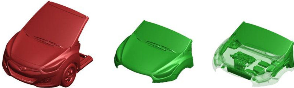
Fig.3: LS-DYNA FE model reduction: full model (left), reduced model (center), deformable parts of the reduced model (right, green transparent).
